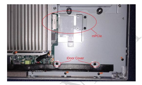
After that you can connect the cables to the mPCIe module and mount the backcover again.
