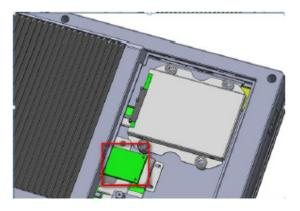
Fix the device with 2 screws.
