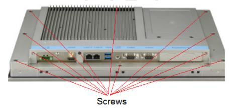
Remove the 2 screws of the iDoor cover and mount your iDoor bracket.
