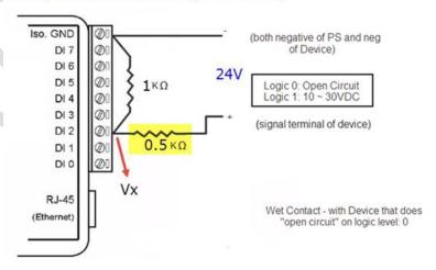
However, we have to emphase that the wiring method is not the standard wiring provided in the user manual, this work around method is only to provide customers convenience when using the sensor with Open and 10~30V wet contact signal, which is not the correct DI spec supported in ADAM-6000.
