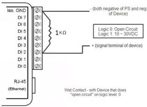
In order to avoid the 1k pull down resistor overheat due to the excessive current, user may also add a current limiting resistor as below picture. The value of current limit resistor and the rated power is based on the current passing through the sensor also the output voltage from the sensor. Take below picture as an example, user can add a 0.5K resistor for a 24V sensor output signal, and the rated power for the extra current limiting resistor should be at least 0.5W.
