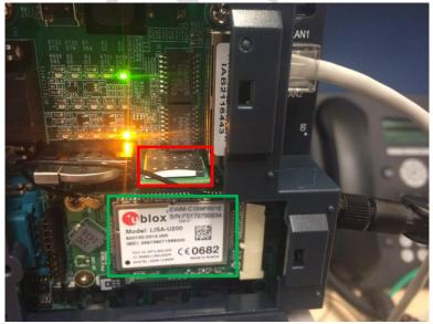
The red block indicates the position where the 3G SIM card is installed. The green block indicates the location of 3G module.
