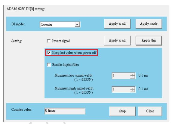
Figure 2. "Keep last value when power off" function
