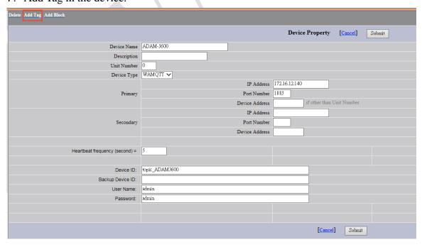
8. Create New Tag with the monitored Tag Name and Address in the device.
