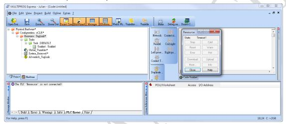
This document explains what port eCLR uses in ADAM-3600. If the port is blocked by the firewall of device, user may not download MULTIPROG project to the device and see the status as timeout.
