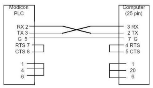
Figure 1.2 RS232-Modicon 984 Cabling Diagram (25 pin COM Port)
