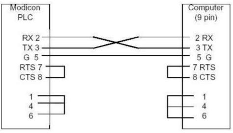
Figure 1.1 RS232-Modicon 984 Cabling Diagram (9 pin COM Port)
