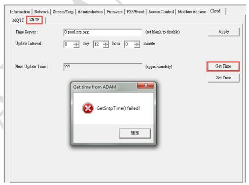
Figure 1 The "GetSntp Time() failed" message on Utility
