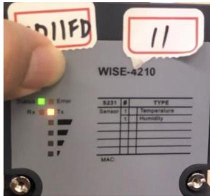
*Figure2. LED status when WISE-4210 transmitting site survey packet*
