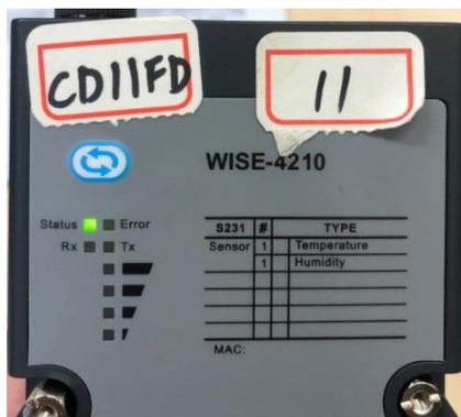
Figure1. LED status when WISE-4210 in site survey mode
