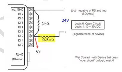
Please note that this wiring method is not standard wiring way provided in the user manual, this work around method is only to provide customers convenience when using the sensor with Open and 10~30V wet contact signal, which does not conform with the correct DI spec supported in ADAM-6000.
