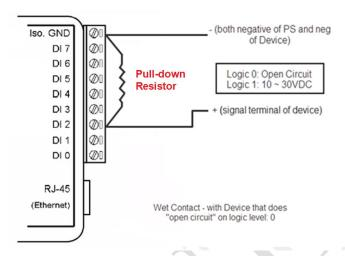
In order to avoid the pull down resistor from overheat due to the excessive current, user may also add a current limiting resistor as below picture. The value of current limit resistor and the rated power is based on the current passing through the sensor also the output voltage from the sensor. Take below picture as an example, user can add a 0.5K resistor for a 24V sensor output signal, and the rated power for the extra current limiting resistor should be at least 0.5W.
