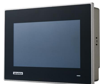
7" Touch Panel Computer with ARM Cortex™-A9 Processor
