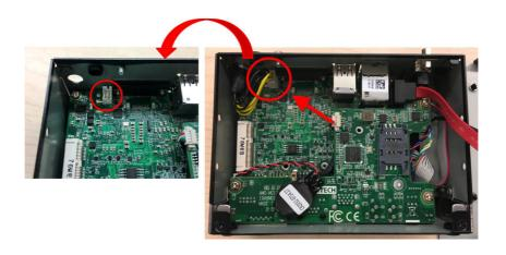
7. Connect power cable between power module and M/B.
