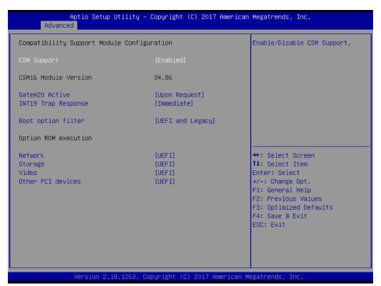
Figure 3.12 CSM Configuration Settings
