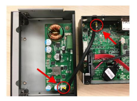
8. Stack ARK plus module with system, and screw two screws each rear side.
