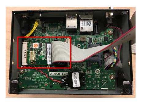
4. Screw I/O plate of iDoor module on ARK Plus module (AMO-1101).
