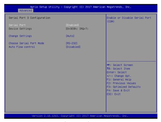
Figure 3.8 Serial Port Settings (Port3)
