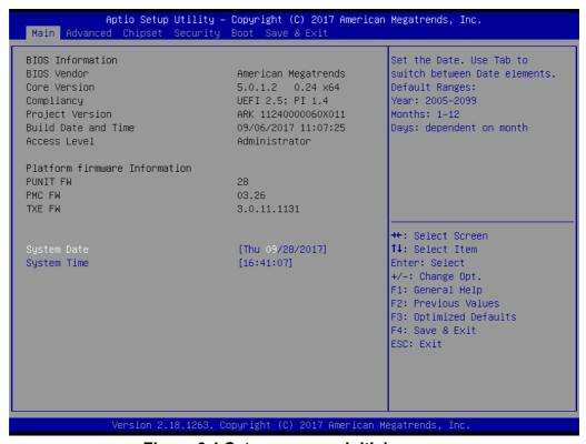
Figure 3.1 Setup program initial screen
