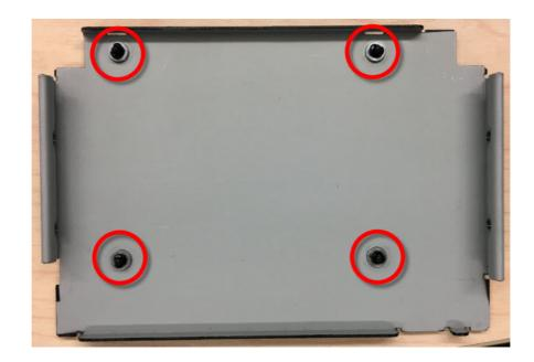
4. Secure 2.5" SATA HDD onto the bottom cover. The screws are in the accessory box.
