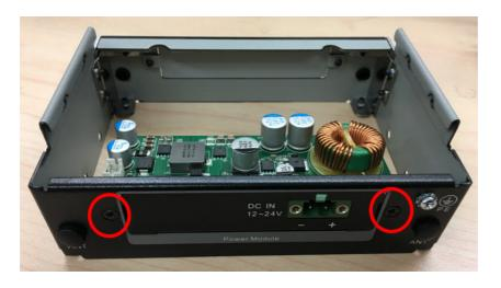
3. Remove the four screws on both sides of ARK-1124.
