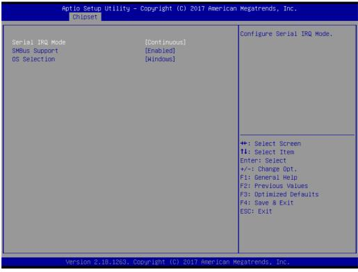
**Figure 3.17 South Bridge Configuration**
