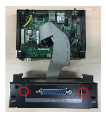
5. Stack ARK plus module with system, and screw two screws on each rear side.
