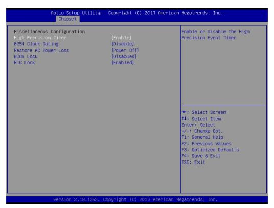
Figure 3.26 Miscellaneous Configuration Settings
