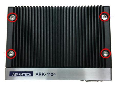
2. Remove the top cover and install the memory into the memory socket.
