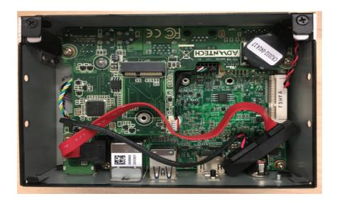
3. Install M.2 module in M.2 slot (position: NGFF\_E\_1) which on the I/O board, then secure module with screw.
