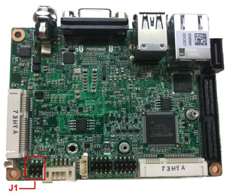
Figure 2.1 Jumper Layout
