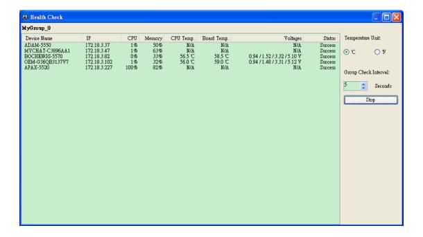
If the field shows "N/A", it means the device does not support that information. The last column "Status" shows the query condition.
