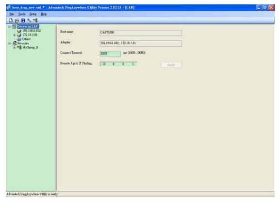
In the right hand side panel, you can modify the "Connect Timeout" value from 1000 to 10000 ms and this value will be applied for all device connections.
