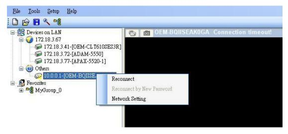
Click on the "Network Setting", you will see a pop up dialog as the left hand side of below. Try to change the network setting, for example, change it to DHCP as the right hand side of below, then press "Apply".
