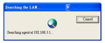
If the IP has no response within "Connect Timeout" value, then the try will go to next IP "192.168.3.2" until a device is found, or reach the last IP "192.168.3.254", or the "Cancel" button is pressed.
