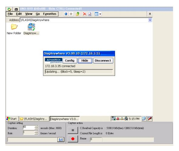
In the "Capture setting" group box, you can setup the "Duration" from 1 to 3600 seconds and the "Rate" for 1 frame or 2 frames per second. And you have to press the
