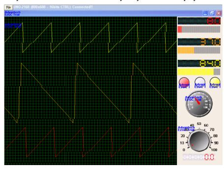
When the "Whole screen firm" is checked, on the utility, you will see the complete screen shot without fragment. **However, this function will consume higher CPU using on the server side**.
