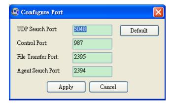
Those ports are used for communicating with server. Before applying the change, you have to change the port setting on the server as well.
