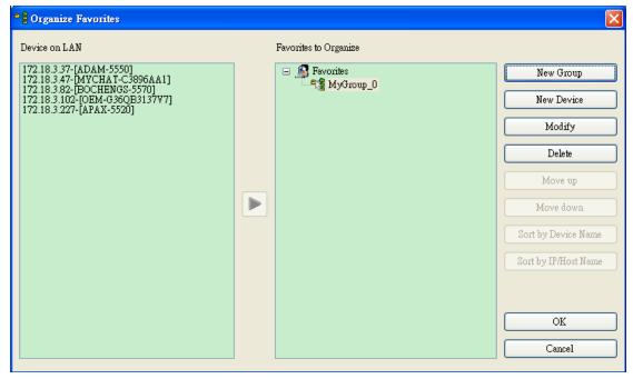
Now, you can press "New Device" to add a new device manually into selected group. Or you can press the "Modify" button to modify to edit the selected group node. Or you can press the "Delete" button to erase the selected group node.
