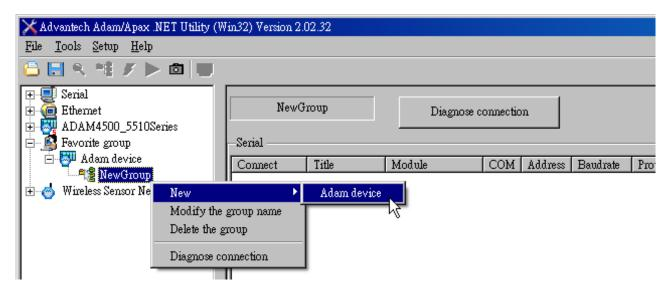
4. Give the device a name and click "Ethernet Device" tab. Fill in the information of connected ADAM device then click "Add."
