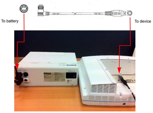
Figure 2.10 Cable connection
