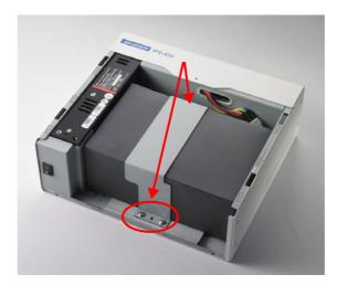
4. Disconnect battery cell cable and system cable to remove old battery cell and replace new one.
