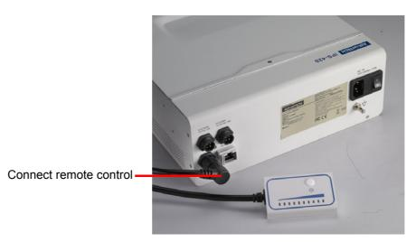
Figure 2.7 Connecting the remote control
