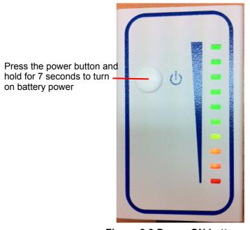
Figure 2.8 Power ON battery
