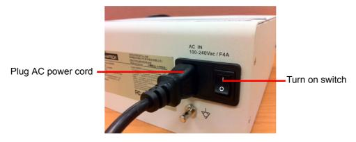
Figure 2.5 AC power cord connecting and power switch on
