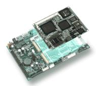
Though small in size, COMs implement CPU architectures and basic common circuits. Many system integrators find that Advantech COM solutions already cover around 80% of their feature requirements. This makes COM products powerful time and cost savers.
