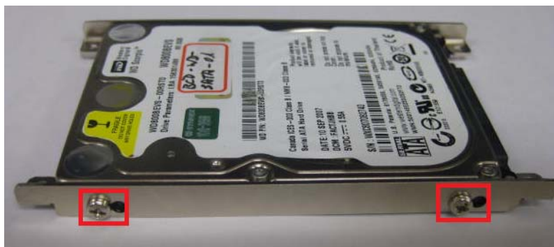
Figure 1.5 Fasten screws on the SATA HDD bracket
