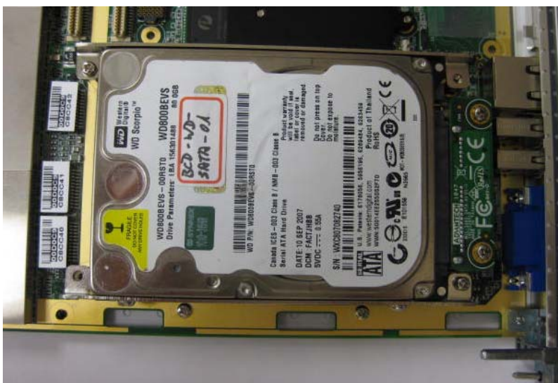
Figure 1.6 Introduce SATA HDD into SATA connector
