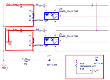
In this way if IDI6 is wet-contacted, the current will flow into the card and the device connect to IDI6 will always be ON if there's not a switch along this way.
