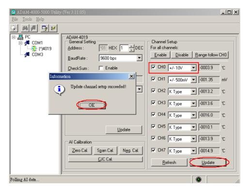
17. Power off the calibrated ADAM-4019 module. Remove the grounded INIT\* pin and then power on the module. Now you have finished the calibration procedures.
