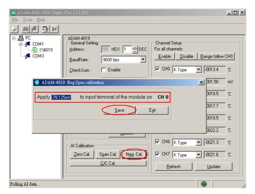
15. For thermocouple input range, it is necessary to adjust CJC temperature by typing in correct CJC offset temperature. Please click "CJC Cal." and type in proper offset of CJC temperature.
