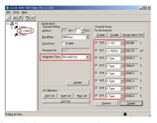
4. Click "Zero Cal." for zero calibration. Apply 0V to CH0 input terminals and then click "Save".
