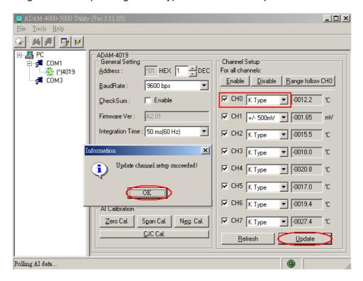
12. Click "Zero Cal." for zero calibration. Apply 0mV to CH0 input terminals and then click "Save".
