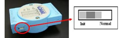
When Initial Mode have been launched, a star sign "\*" after ADAM model name will also be shown while performing search. That indicate user that the Initial Mode have been successfully launched and may proceed modifying "Modbus RTU" protocol.
