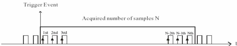
**Figure 4.1: Post-Trigger Acquisition Mode**
