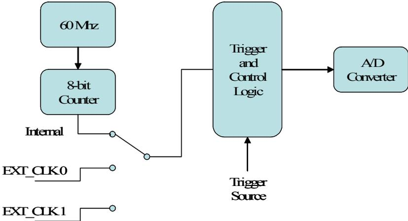
*Figure 4.5: MIC-3714 Sample Clock Sources*
