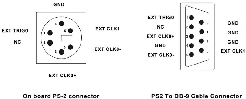
**Figure 3.3: I/O Connector Pin Assignment**
