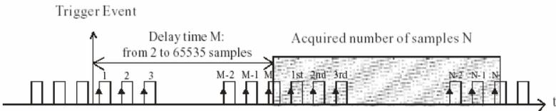
**Figure 4.2: Delay-Trigger Acquisition Mode**
