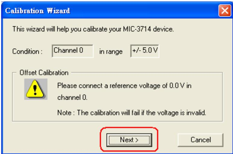
**Figure 5.3: Start-up Window for Offset Calibration**
