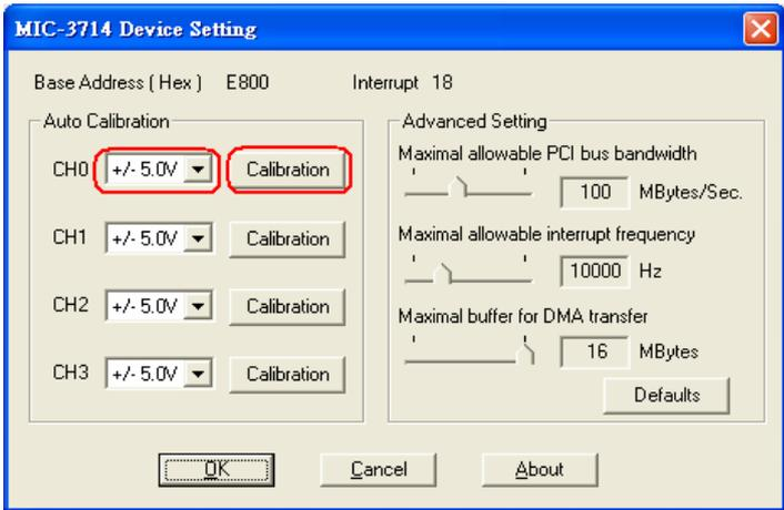
**Figure 5.2:** Calibration Button launches Calibration
