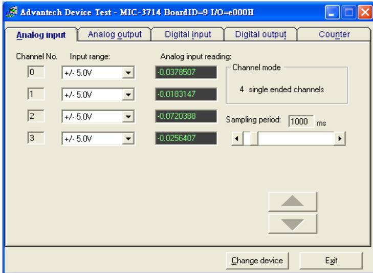
*Figure 2.5: Device Test Dialog Box*
