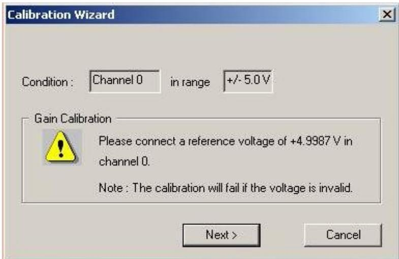
**Figure 5.7: Start-up Window for Gain Calibration**
