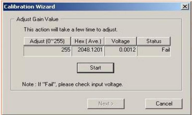
**Figure 5.10: Gain Calibration Failed**
