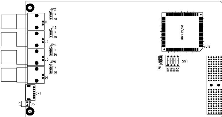
*Figure 3.1: Connector, Jumper, and Switch Locations*
