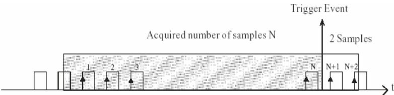
**Figure 4.4: Pre-Trigger Acquisition Mode**
