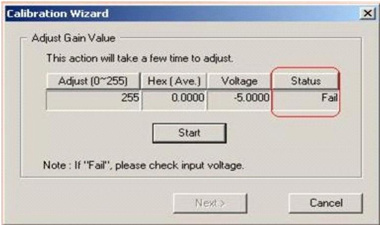
**Figure 5.6: Offset Calibration Failed**
