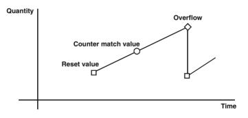
Figure 3.3: Example for counter operation
