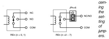
Figure 4.1: Relay structures and connections
