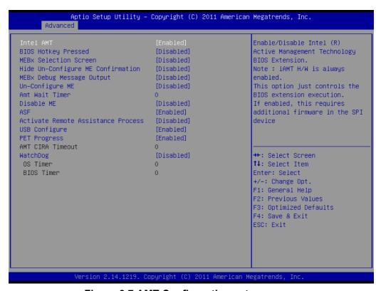
Figure 3.7 AMT Configuration setup screen
