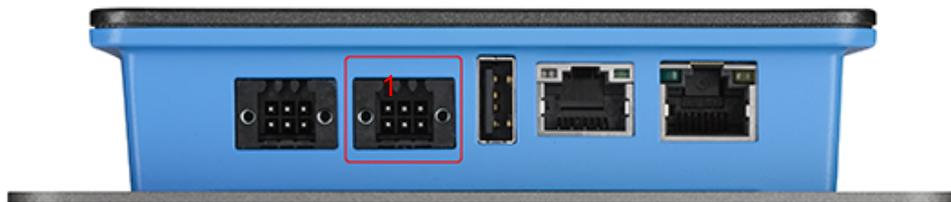
Figure 2.9 GPIO connector
