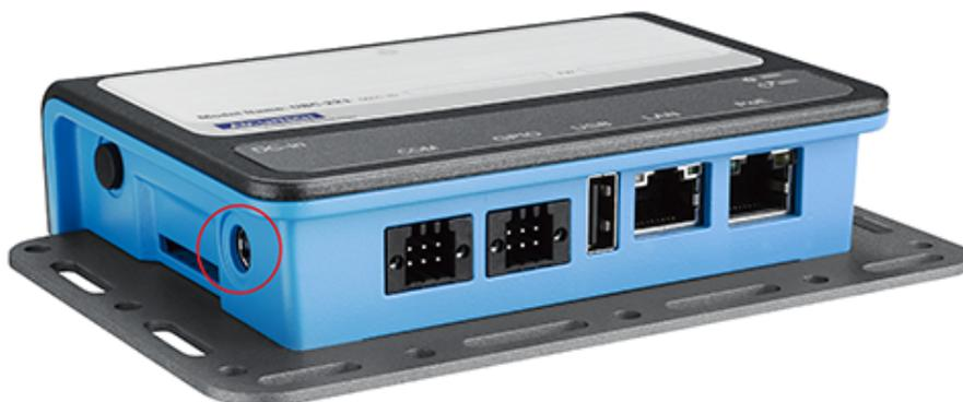
Figure 2.4 Power input connector
