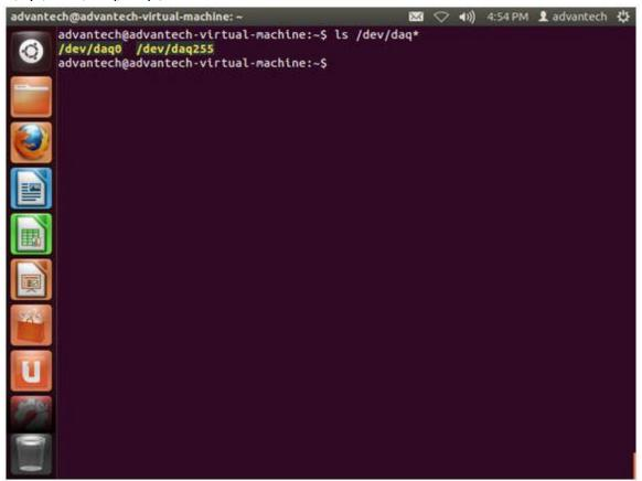
4. Finally, make sure the DAQ device node has read and write permissions.
