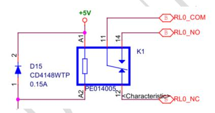
In general, the relay has three pins, COM, NO and NC. NO means when a relay doesn't power on, the output circuit is open. NC means when a relay doesn't power on, the output circuit is close. If a module support the Form C, the customer can choose Form A and Form B. Form A is connecting the loading device to RLx\_COM and RLx\_NO. Form B is connecting the loading device to RLx\_NC.
