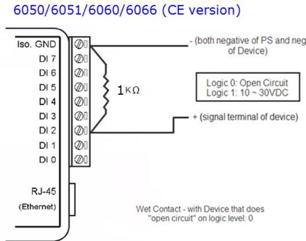
In order to avoid the 1k pull down resistor overheat due to the excessive current, user may also add a current limiting resistor as below picture. The value of current limit resistor and the rated power is based on the current passing through the sensor also the output voltage from the sensor. Take below picture as an example, user can add a 0.5K resistor for a 24V sensor output signal, and the rated power for the extra current limiting resistor should be at least 0.5W.
