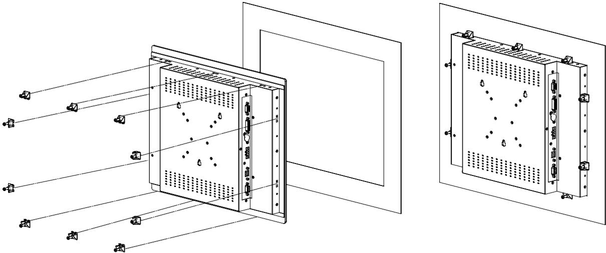
Figure 2.2 Panel Mounting (392 x 292 mm)
