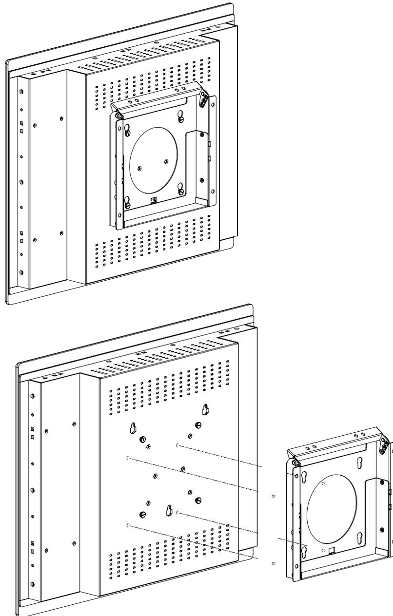
Figure 2.1 Wall Mounting for FPM-8151 Series
