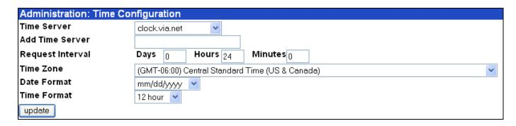
From here you can set the time configuration used for time stamping on the 102RAS. You can make modifications then click the update button to save the new configuration.
