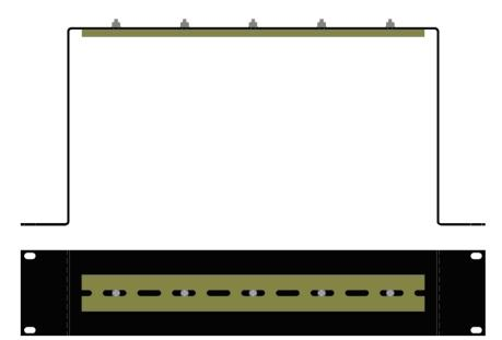
Most N-Tron<sup>TM</sup> products are designed to be mounted on industry standard 35mm DIN rail. However, DIN rail mounting may not be suitable for all applications. Our Universal Rack Mount Kit (P/N: URMK) may be used to mount the 102RAS to standard 19" racks as an option.
