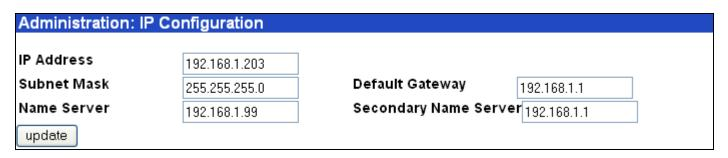
You may change the values to apply to your network and select the update button to save the values. The fields for "IP Address", "Subnet Mask", "Default Gateway" and "Name Server" are required. A "Secondary Name Server" is optional.
