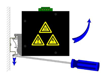
To mount the unit to the 35mm DIN rail, place top edge of the brackets on the back of the unit against the DIN rail at a 45° upward angle. Lower the bottom of the unit until it snaps into place on each bracket.
