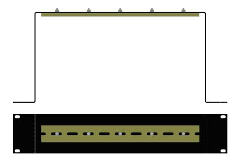
Most N-Tron<sup>TM</sup> products are designed to be mounted on industry standard 35mm DIN rail. However, DIN rail mounting may not be suitable for all applications. Our Universal Rack Mount Kit (P/N: URMK) may be used to mount the 105TX/FX-POE enclosures to standard 19" racks as an option.
