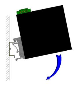
To install the unit to 35mm industrial DIN rail, place the top edge of the included mounting bracket on the back of the unit against the DIN rail at a 15° angle as shown. Rotate the bottom of the unit to the back (away from you) until it snaps into place.
