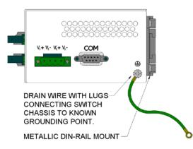
If the use of shielded cables is required, it is generally recommended to only connect the shield at one end to prevent ground loops and interfere with low level signals (i.e. thermocouples, RTD, etc.). Cat5e cables manufactured to EIA-568A or 568B specifications are required for use with N-Tron Switches.
