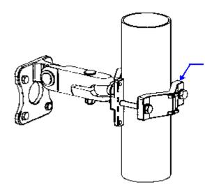
Bracket orientation for larger (up to 3" [76mm] dia.) pipe
