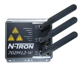
The N-TRON 702-W Industrial Ethernet Wireless Device offers outstanding performance and ease of use. It is ideally suited for connecting wireless devices to a wired network and connecting two wired networks together where wires are not possible or practical to be installed.
