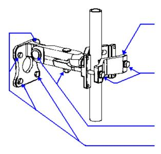
Bracket orientation for small (1" [25mm] dia.) pipe
