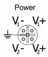
The M12 A coded power connector is keyed, where the mating connection from the power supply can be made only when the male and female ends are lined up properly. Verify the Power LED stays ON (GREEN).
