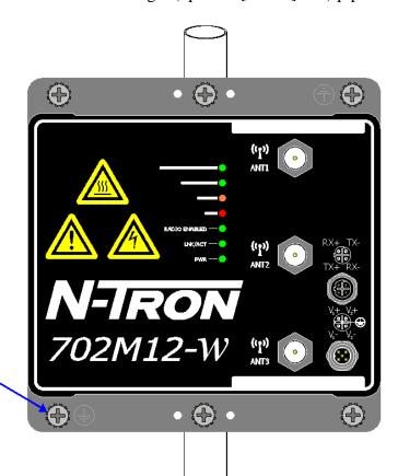
6x Tighten #10-32 screws until split lock washers fully compress (all installations)
