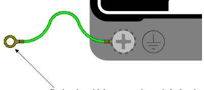
Drain wire with lug connecting switch chassis to known grounding point.
