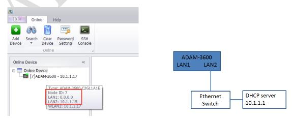
Note: If LAN port is not connected with any devices, the default IP will be 0.0.0.0.
