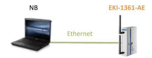
Step 1: Connect the EKI-1361 via Ethernet cable
