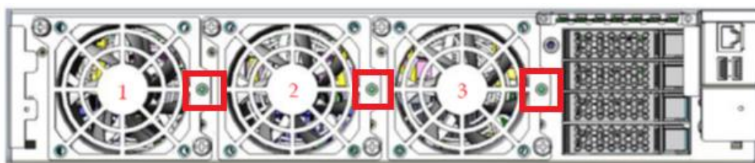
Figure 18: Fan LED location
