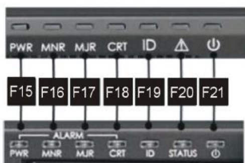
Figure 34: The locations of LEDs
