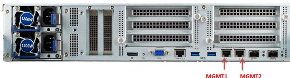
Figure 3: The Location of Management Ports at Rear Panel
