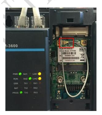
The primary RF interface (ANT1), indicated in red square, supports both TX and RX, providing the main connection of antenna. If the user only has one antenna, connecting ANT1 could make it normally.
