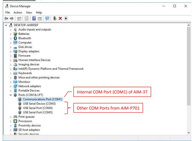
3. When un-dock AIM-37 from AIM-P701, <u>Device Manager</u> should automatically refresh to make <u>Ports(COM & LPT)</u> remain only <u>internal COM Port (COM1)</u> as initional status.
