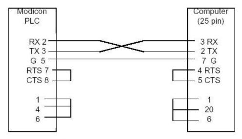
Figure 2 RS232 - Modicon 984 Cabling Diagram (25 pin COM Port)
