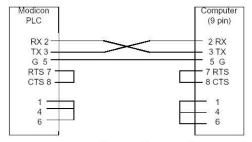
Figure 1 RS232 - Modicon 984 Cabling Diagram (9 pin COM Port)
