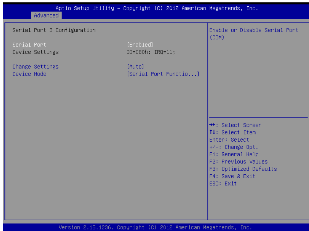
Figure 3.21 Serial Port 3 Configuration
