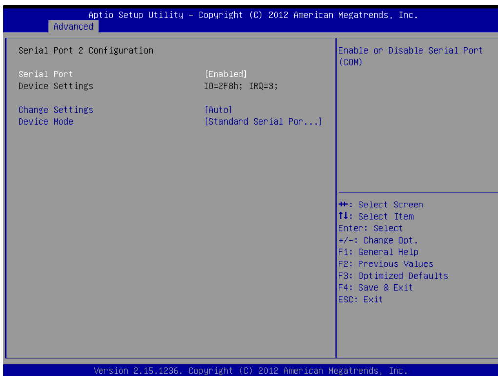
Figure 3.17 Serial Port 2 Configuration
