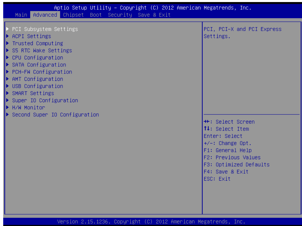
Figure 3.3 Advanced BIOS features setup screen
