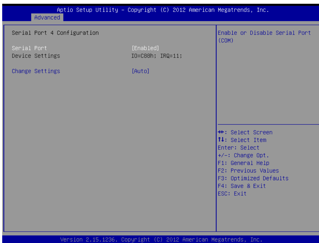
Figure 3.22 Serial Port 4 Configuration
