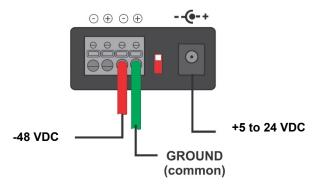
**NOTE:** When using stranded wire, the leads must be tinned, and equivalent to a 16 AWG solid conductor. The IE-Giga-MiniMc TX/SFP is protected against mis-wiring; If mis-wired, the IE-Giga-MiniMc TX/SFP will not function. The IE-Giga-MiniMc TX/SFP is internally connected to the negative DC power terminals.
