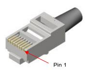
NOTE: MDI/MDIX AutoCross function will automatically transpose the Transmit and Receive lines if required.
