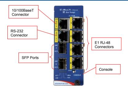
The IE-iMcV-E1-Mux/4 includes a console serial port. To establish a link between a module's console port and a local PC, connect the Mini Jack to DB9 adapter that is included with the B+B SmartWorx. This serial console port connection provides access to the IE-iMcV-E1-Mux/4 module CLI configuration screens. Set the computer/terminal for VT-100 emulation, 38.4K baud, 8 data bits, 1 stop bit, no parity and no flow control. Under the VT-100 emulation, set the backspace key to send delete.
