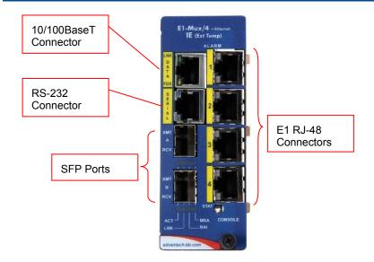
The IE-iMcV-E1-Mux/4 features diagnostic LEDs as explained below.
