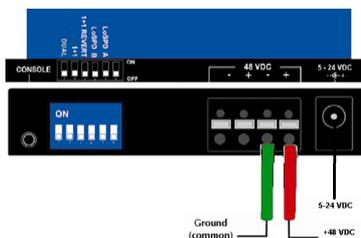
**NOTE:** When using stranded wire, the leads should be tinned. The DC terminal block is protected against polarity mis-wiring. AWG24 is recommended.
