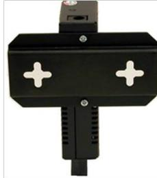
The IE-MultiWay can be mounted with two DIN rail clips, (available from B+B SmartWorx). The DIN rail clips include screws to allow the installation on a DIN rail. Install the screws into DIN rail clips (can be mounted parallel or perpendicular to the DIN rail). Snap the converter onto the clips. To remove the converter from the DIN rail, use a flat-head screwdriver into the slot to gently pry the converter from the rail.
