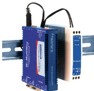
**SHOWN:** IE-MultiWay with optional DIN rail mount power supply.
