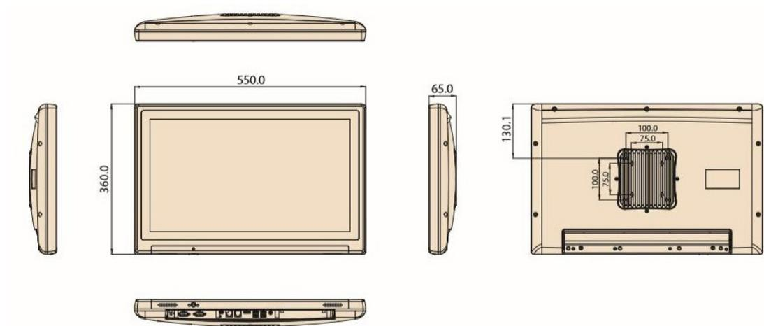
**Figure 1.1 Dimensions of the POC-W213L Series**
