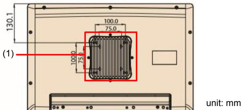
Figure 2.2 Rear view of the Point of Care Terminal
