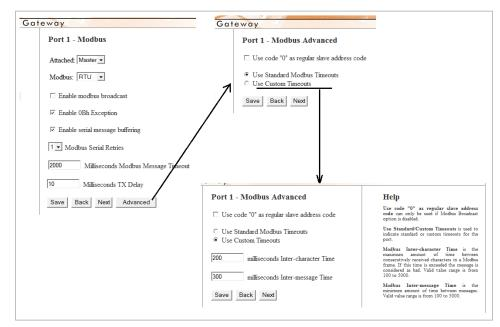
Figure 33. Modbus Port Screen Advanced
