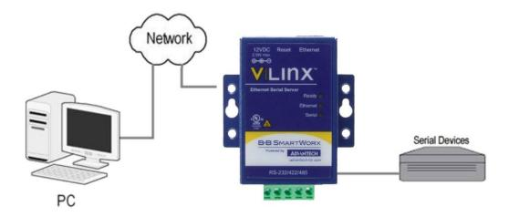
Figure 43. Direct IP Connection
