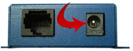
Figure 9. BB-MESP211 Power Connection
