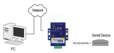
Figure 11. BB-MESP211T Connections
