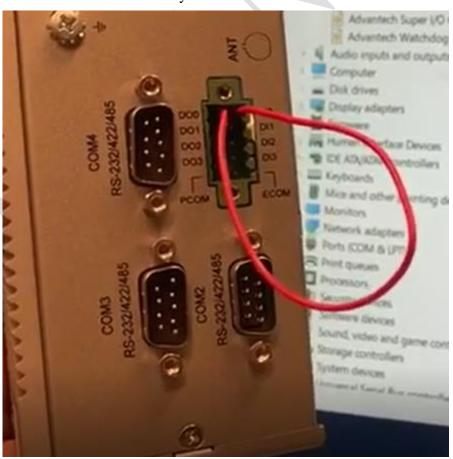
2. Open the ADVGPIOTool and set the GPIO4 as low. The GPIO0 will light up.
