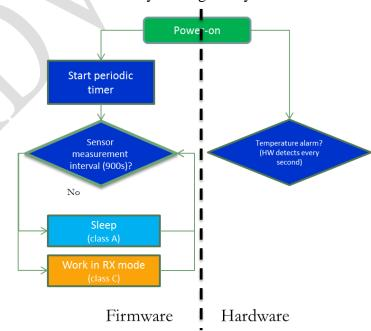
Figure. Work flow chart of WISE-2410 firmware.
