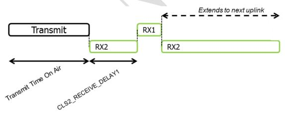
Class C end-device reception slot timing.
