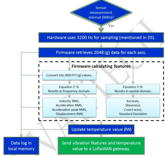
Figure. Work flow chart of WISE-2410 firmware.
