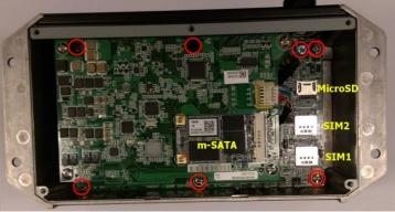
Figure 3.1 install peripheral in the system
