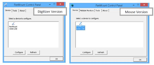
Take the PenMount 6000 for example, the device configuration window will appear after clicking on the "PenMount 6000 USB" or "PenMount 6000 RS232" icon in the PenMount Control Panel.
