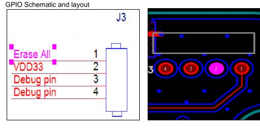
• Open pin1 and pin2 (or pin1 remains 0V) → Quick Erase disabled or Write Protect disabled
