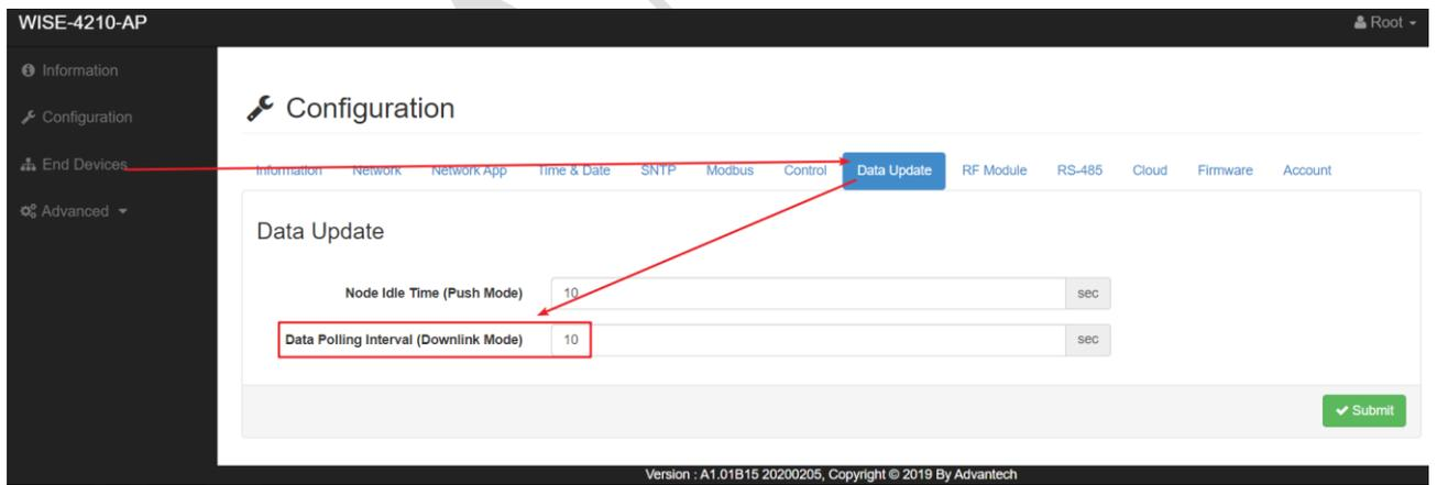
Figure4. Configuration of Polling Interval for Downlink Mode
